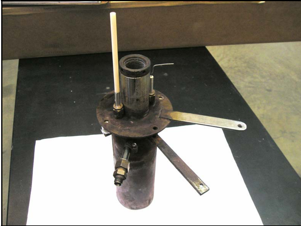
Figure 2. Direct Carbon Fuel Cell (DCFC) Apparatus Tested at WVU.
