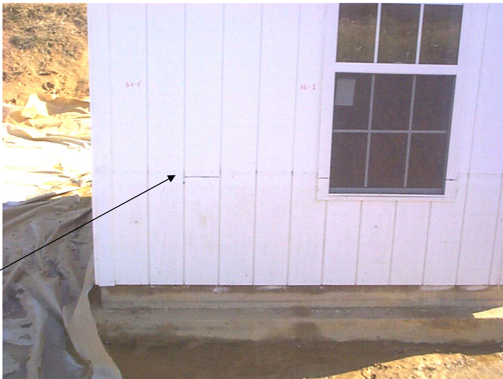
Figure 4-14 Module S-1 (Wall 1, North Exterior Wall) Post-flood, Day 4. Walls are stained below flood level.
