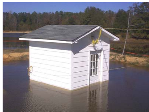
Figure 4-1 (Left) Module S-1 (Slab-on-Grade Unit) during flooding. The arrow shows the sensor cables coming from the attic.
