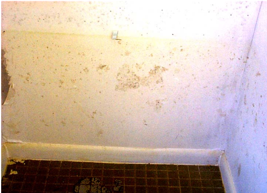
Figure 5-11 Module C-2 (Wall 2) Day 10 after washing with water. Staining and mold growth remain
