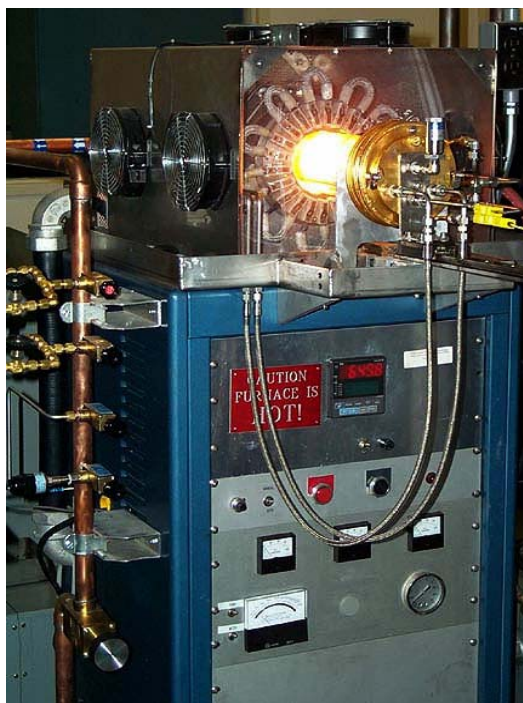
Fig. 1. ORNL's circular infrared furnace used to heat the parts after they were coated with zirconia-based solution.
