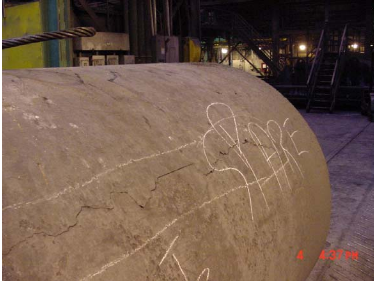
Fig. 1. Coiler drum showing large cracking running along outside surface.
