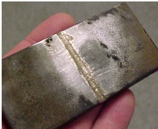
Fig. 2. Photograph showing a butt joint in ~ 9-mm-thick die material made by torch-brazing with BAg-7 filler metal.
