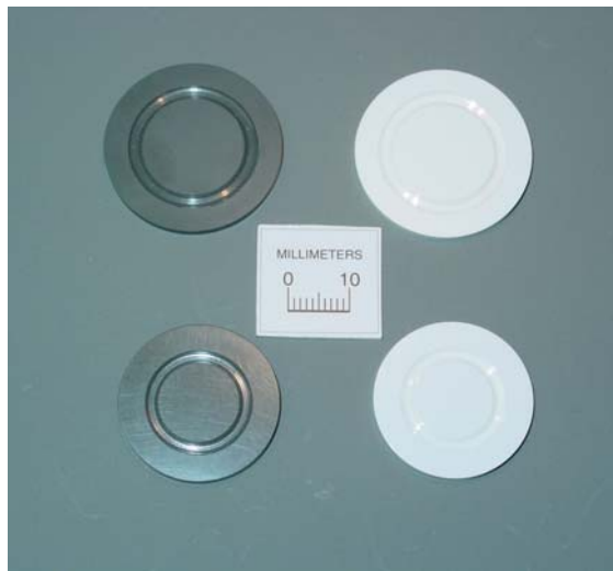
Fig. 1. Machined seal disks made of ceramic material. The disks on the left are made of \text{Si}_3\text{N}_4 , and the disks on the right are made of \text{ZrO}_2 .
