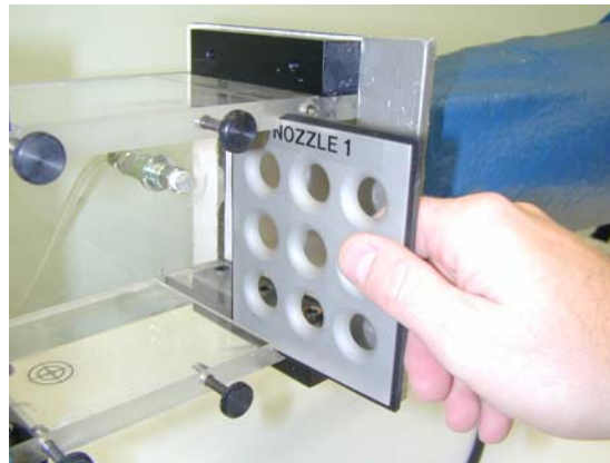
Figure 3. Nozzle Plate for Creating Low Velocities
