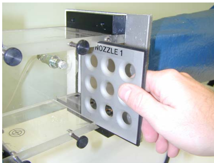
Figure 12. Correct Installation of a Nozzle Plate
