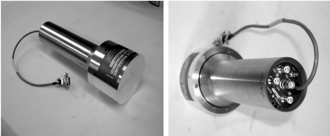
Fig. 11. The FMFM gamma ray detector is a commercially available BGO scintillation detector (on the left) with a preamplifier, as shown from the top on the right.
