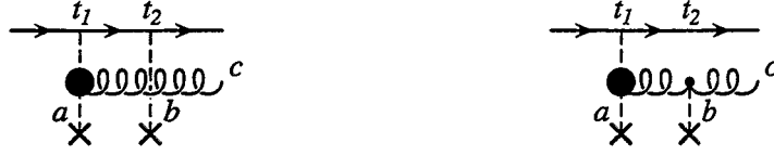
FIG. 1. Rescattering at t_2 of the initial quark and of the secondary gluon produced at t_1 .
