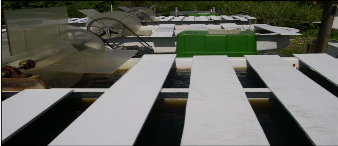
Intermittently Illuminated Raceway Pond, 33% Open Area (15cm wide slat, 7.5cm wide gap)
