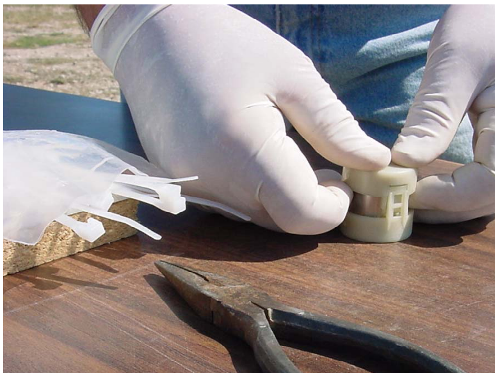
Figure 3. Accu Core Sampler Being Sealed
