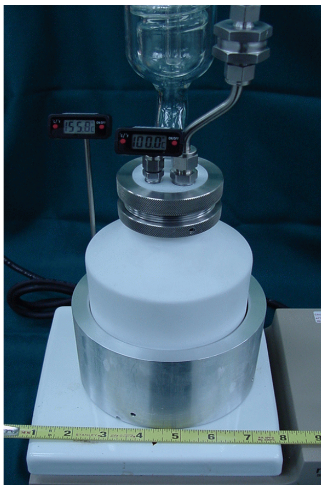
Fig. 4.2. Photograph of dissolver used for pellet dissolution.
