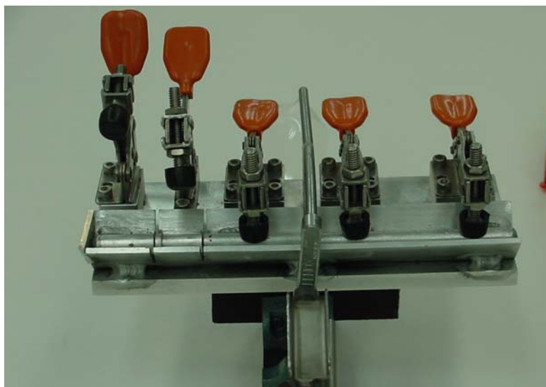
Fig. 4.1. Photograph of stainless steel saw jig used to section targets.
