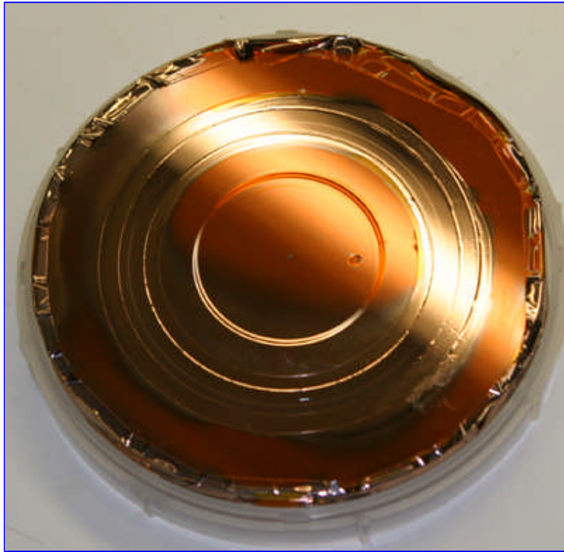
Disk masked with Kapton tape after sputtering 3-5 \mu\text{m} of Cu
