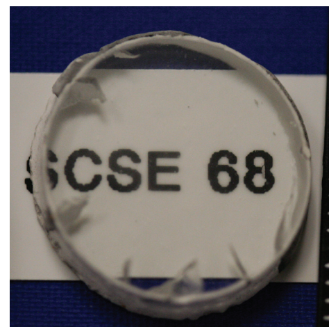
Livermore researchers have produced 15-millimeter-diameter samples of transparent ceramic yttrium–aluminum–garnet. A sample exhibits excellent optical qualities after hot isostatic pressing (right).
