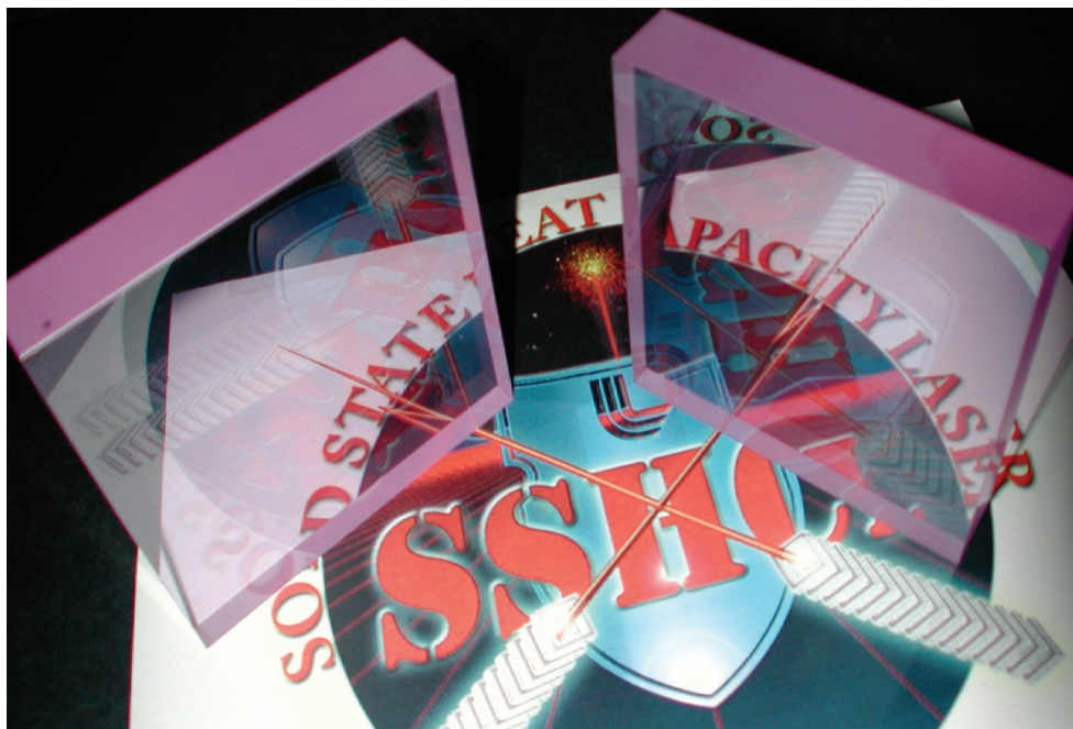
The SSHCL uses the world's largest laser-quality transparent ceramic amplifier slabs, which measure 10 by 10 by 2 centimeters.
