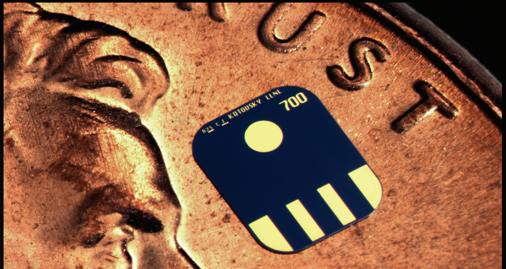
One stress sensor measures just 4 millimeters square and 50 micrometers thick.
