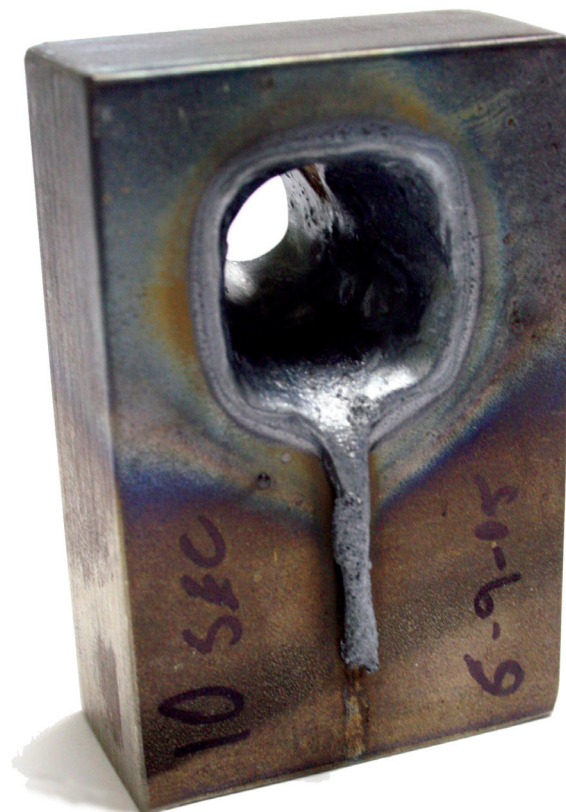
The SSHCL can penetrate a 2.5-centimeter-thick piece of steel in 2 to 7 seconds. In the sample shown, the time span of the entire shot was just 10 seconds.
