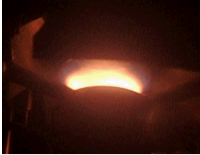
FIGURE 2. Photograph of the discharge above the substrate when the pressure of the Ar/H 2 gas mixture is 150 Torr
