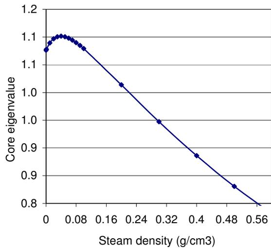
Figure 2: Core Multiplication Factor vs. Steam Density
