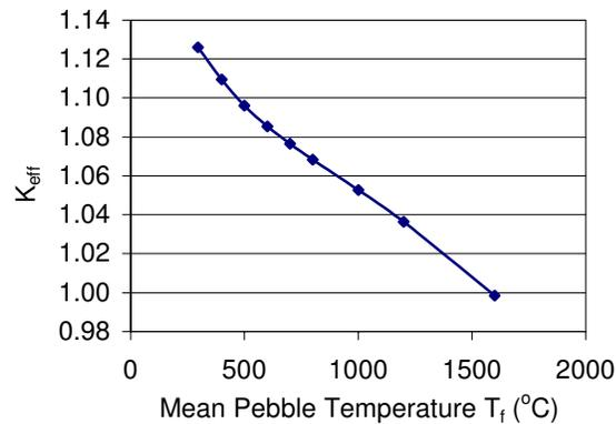
Figure 3: Core Multiplication Factor vs. Average Fuel Temperature
