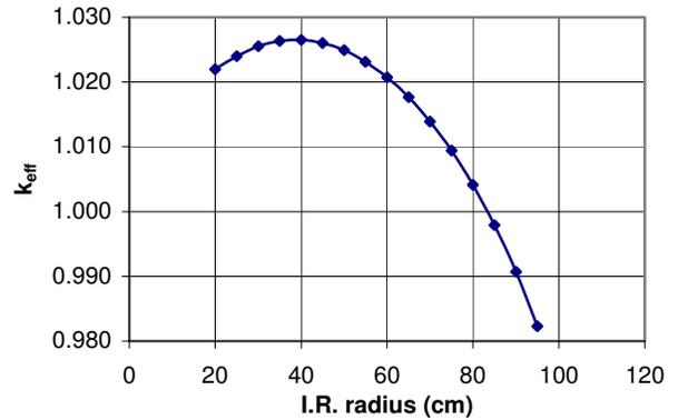
Figure 1: Asymptotic Core Eigenvalue vs. Radius of Inner Reflector – VHTR-300
