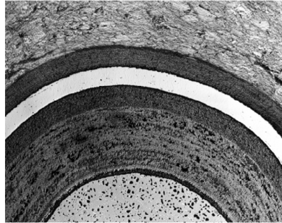
Figure 13. Photomicrograph of German AVR fuel after irradiation.
