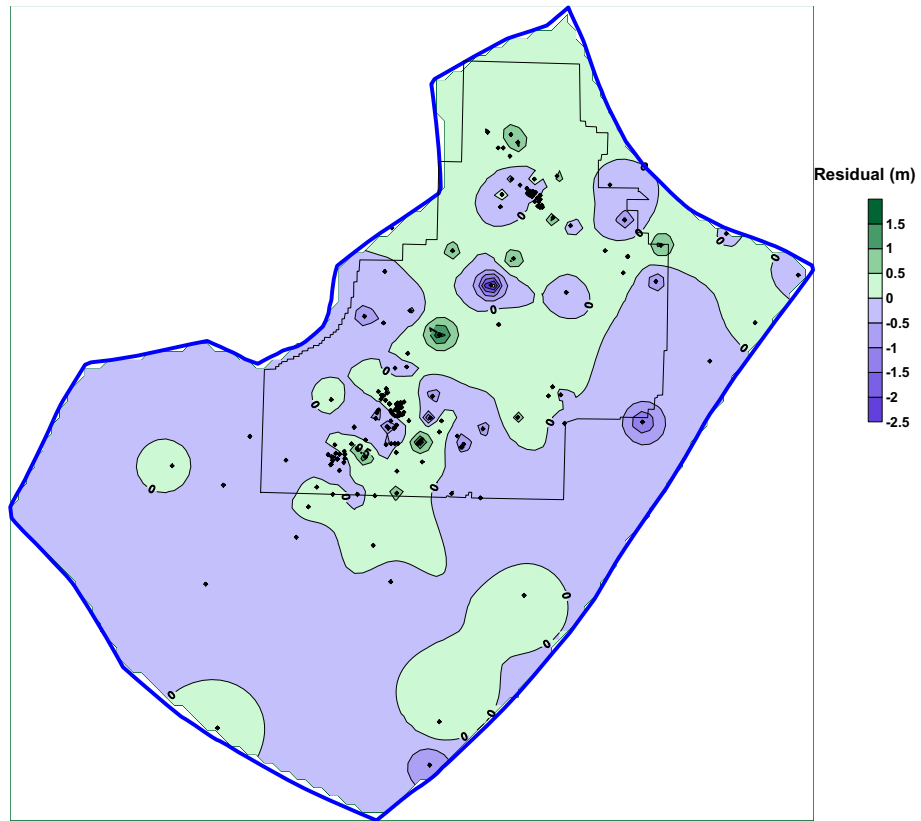
Figure 4-13. Head residuals (simulated minus observed) for all model layers, thick scenario, calibrated with pilot point approach using sedimentary layer bounds (base case model 2).
