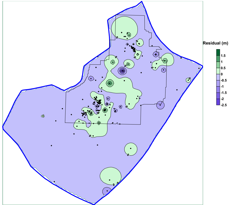
Figure 4-8. Head residuals (simulated minus observed) for all model layers, thick scenario, pure pilot point calibration (base case model 1).
