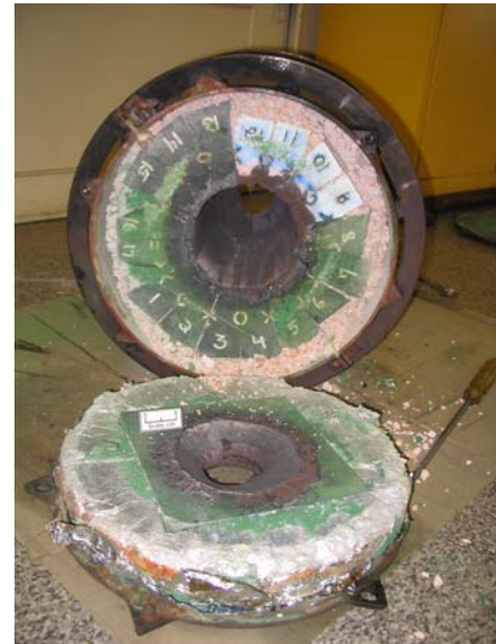
Figure 3 – Chrome and non-chrome based refractory samples tested for molten slag resistance in the rotary slag test. Test conditions included 4 hours of exposure to a coal gasifier slag at 1667°C.
