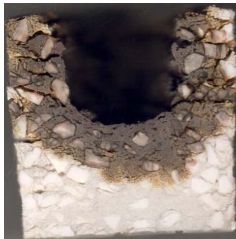
Figure 2. An example of large cup test to evaluate refractory/slag interaction and slag penetration at 1600°C in air.
