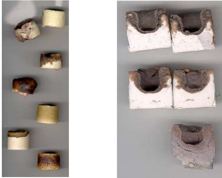
Figure 1. Small “cup” tests conducted to evaluate refractory/slag interactions at 1600°C in an Ar atmosphere.
