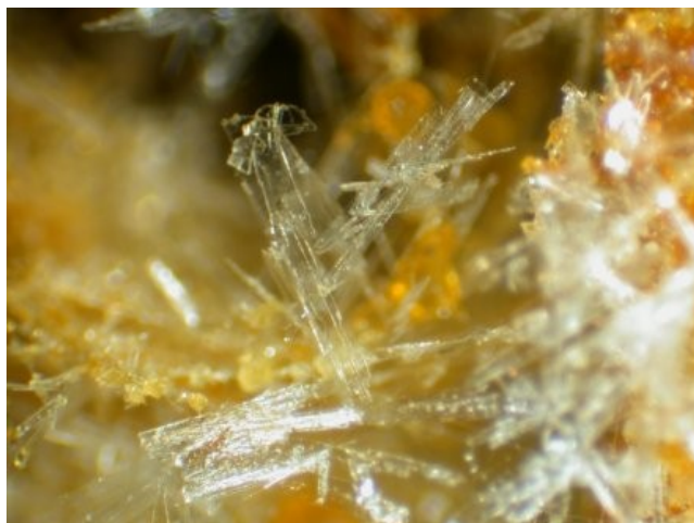
Figure 6. Digital photograph of N, N'-bis(2-hydroxyethyl) ethylenediamine crystals recovered after thermal regeneration of IAS at 120°C.
