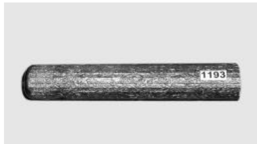
Fig. 2 Smooth ingot surface melted with 0.5 weight percent slag.
