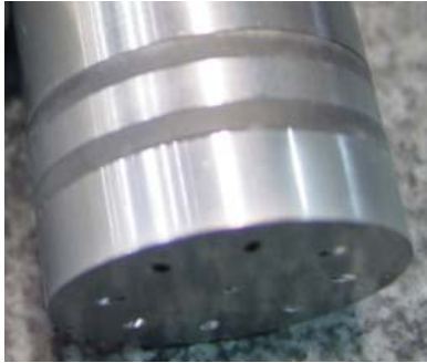
Figure 3: Photograph of the centerbody with attached CCADS electrodes.
