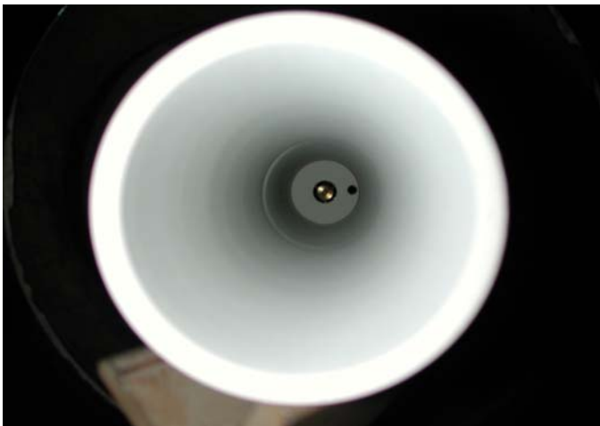
Figure 3. View from the combustor exhaust, showing the white thermal barrier coating on the combustor wall. Pilot flame inlet is to the right of the premixer inlet.
