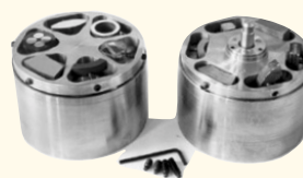
The original specimen holders, especially made for SKF Steels samples
