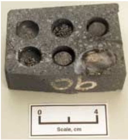
Figure 1a: Refractory brick drilled for reaction with slag components
