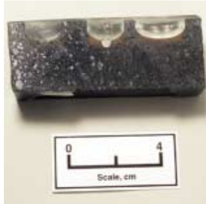
Figure 1b: Cross-section of the drilled refractory brick after thermal treatment and backfill with epoxy
