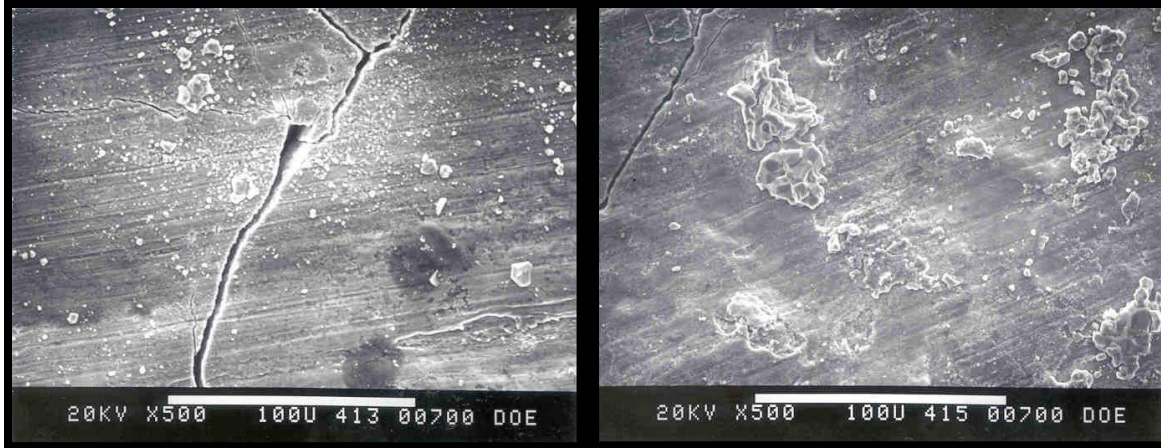
Figure 6. Pictures showing corroded (on left) and eroded-corroded (on right) surfaces of 2 ¼ Cr 1 Mo steel after exposure at 600°C in simulated gasifier gas for 120 hrs.
