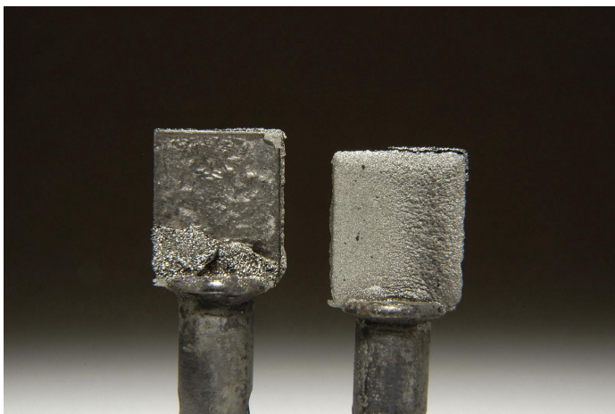
Figure 3. 2 ¼ Cr 1 Mo steel after HAET test at 600°C and 20 m/sec. Corrosion sample is on the left and the erosion-corrosion sample is on the right.
