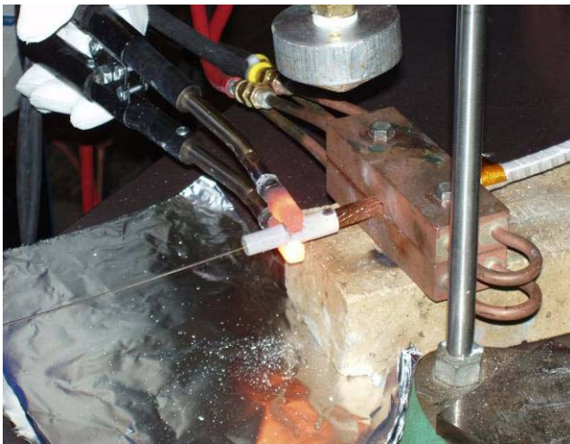
Figure 10- Brazing of Conductor Leads
