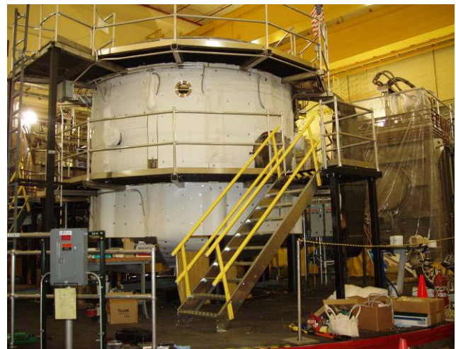
Figure 8- Autoclave used for VPI of Modular and TF Coils
