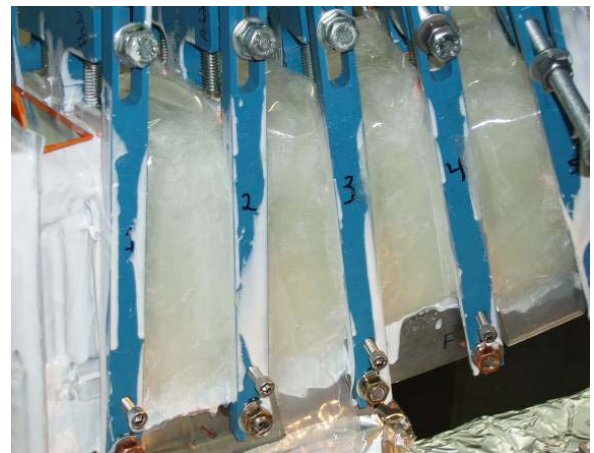
Figure 12 – Epoxy Shell Mold
