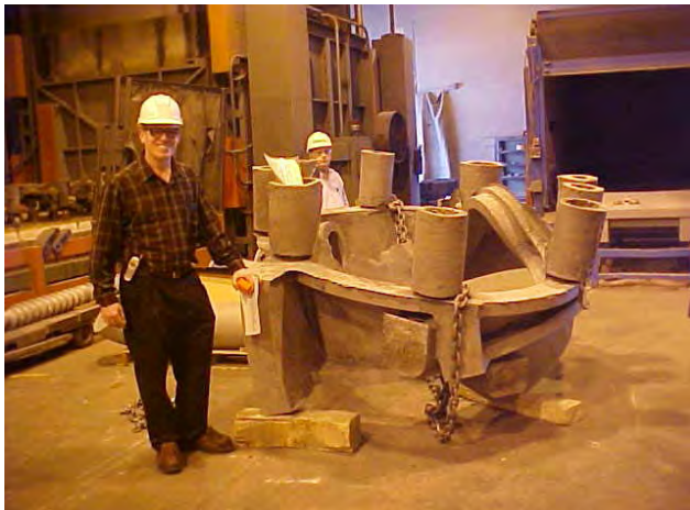
Figure 6. A Casting After Shakeout
