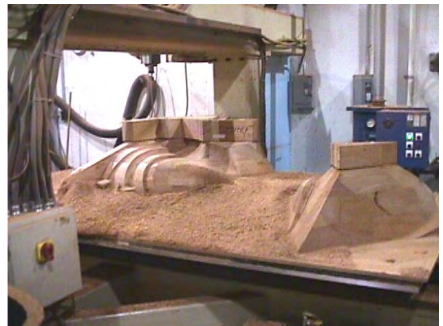
Figure 4. Contour Milling of a Pattern
