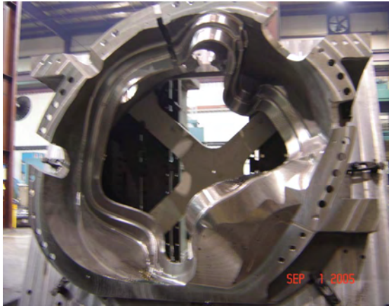
Figure 8. A Casting During 3-Axis CNC Machining
