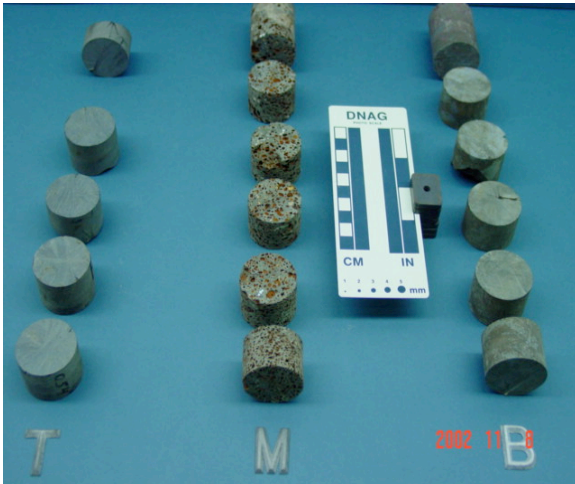
Figure 3. Sectioned core from CRBG T: top, cap rock; M: middle, flow top zone; B: bottom
