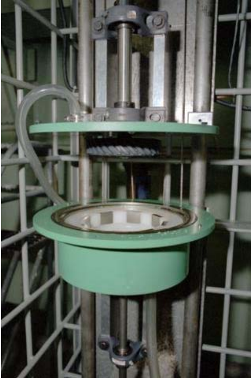
Figure 2. Open slurry erosion/corrosion test apparatus
