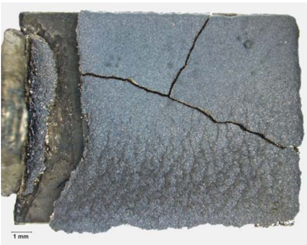
Figure 4. The 9 Cr 1 Mo sample after testing at 700°C. The thick fragile upper scale is partially removed exposing the next layer of scale.
