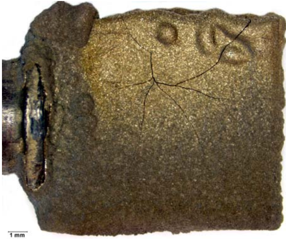
Figure 5. Waspaloy sample eroded at 700°C in a gasifier environment. Specimen shows cracking emanating from the erosion/corrosion zone.
