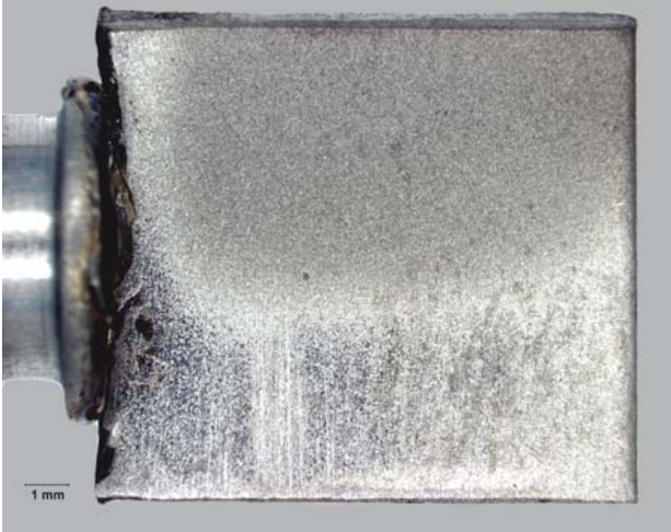
Figure 3. . A Waspaloy sample after room temperature testing that shows the typical roughing of the surface during testing.
