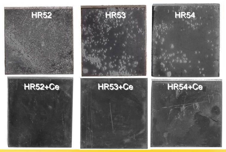
Oxidation Resistance of 9-12%Cr Steels: Effects of Rare Earth Surface Treatment
