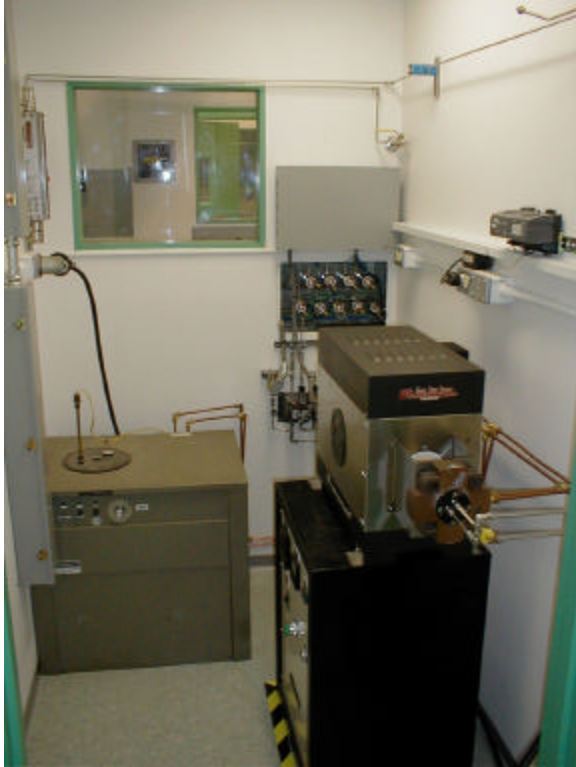
Fig. 6. Tube furnace and module for oxidation in a temperature gradient.
