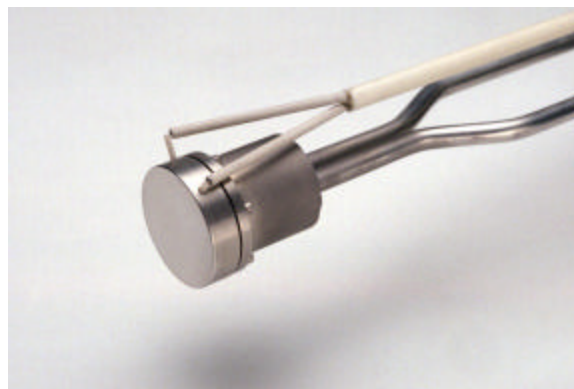
Fig. 4. Sample assembly with a machined cobalt disk with internal thermal couples and attached to an air-
