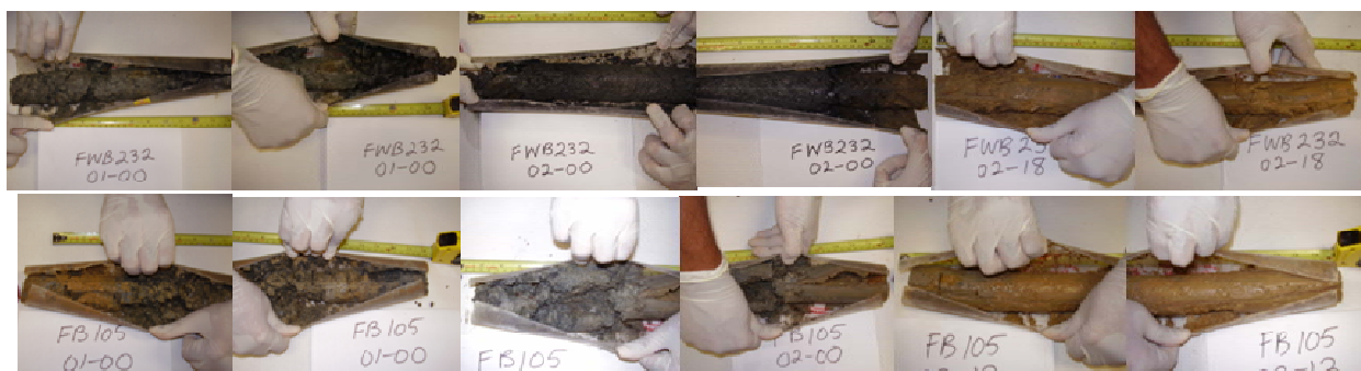
Fig. 8. Photos of sediment in the vicinity of the gravel layer at Area 2 from cores collected within (FWB232; upper set) and outside of (FB105; lower set) the zone of biostimulation at the end of the in situ biostimulation experiment. Note the distinct darkening of materials in the biostimulated sediments, which is indicative of Fe(III) oxide reduction activity.
