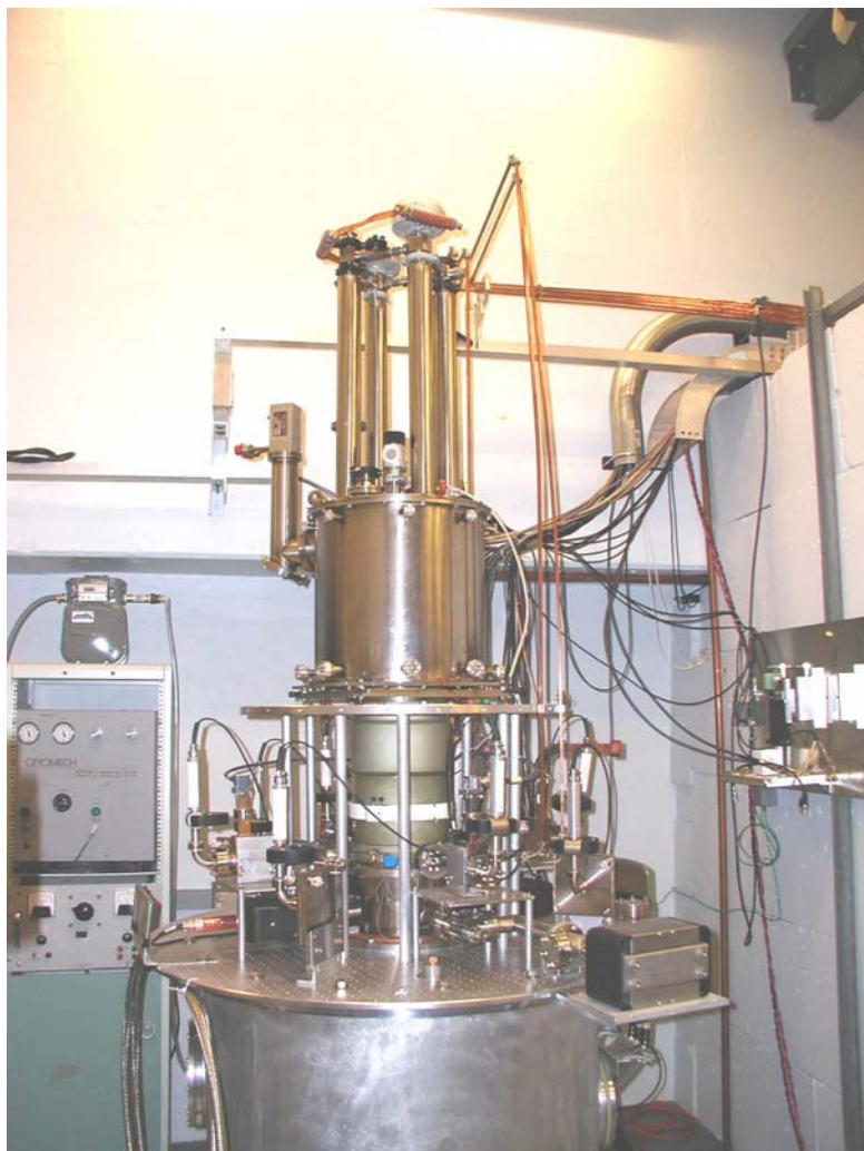
Figure 1. A general view of the 34.3 GHz magnicon.
