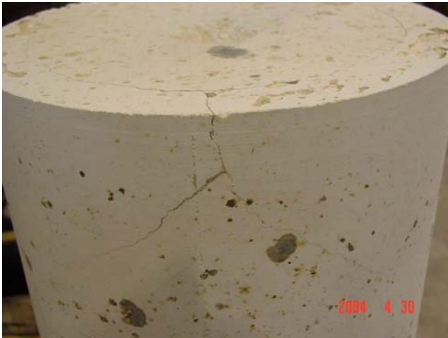
Figure 3: An example of conditions typically observed on many crucibles after testing is shown above (note the cracks). The dark spots were simply “discoloration” from an unknown source and not evidence of metal penetration.
