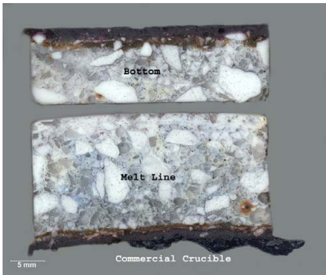
Figure 7: Photomacrograph of the core sample cross sections are shown above. No evidence of erosion of the crucible was observed. Note that the back side of the bottom sample had been cut off to facilitate mounting.
