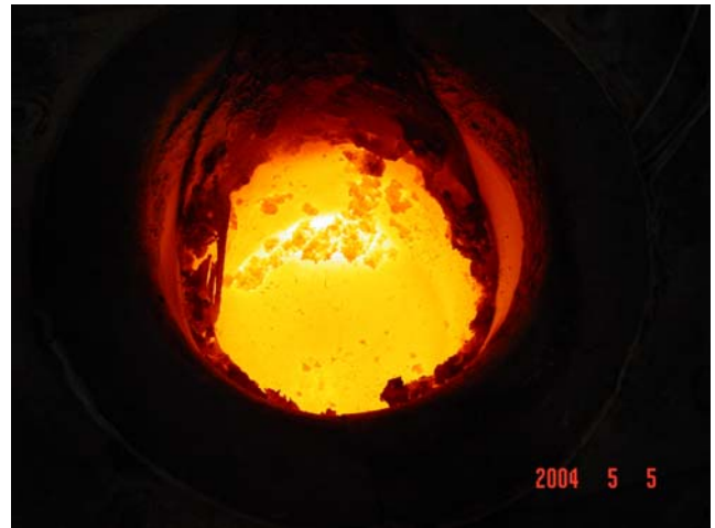
Figure 2: An example of a test crucible is shown above after pouring off the heat. Note the heavy dross left at the melt line.
