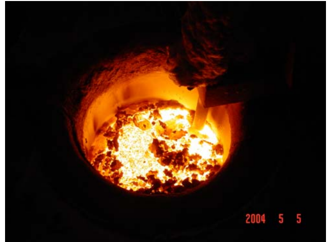
Figure 1: Example of the typical appearance of the melt is shown above. Note the dross (darker material inside the crucible) that remained on the surfaces of the melts for the majority of each of the tests. The immersion thermocouple used to monitor and control the bath temperature is also evident in the photo.
