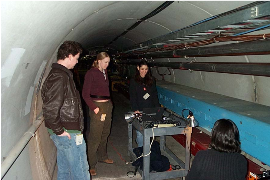
Figure 2 Cart and laptop the digital level is in the lower right hand corner of the picture
