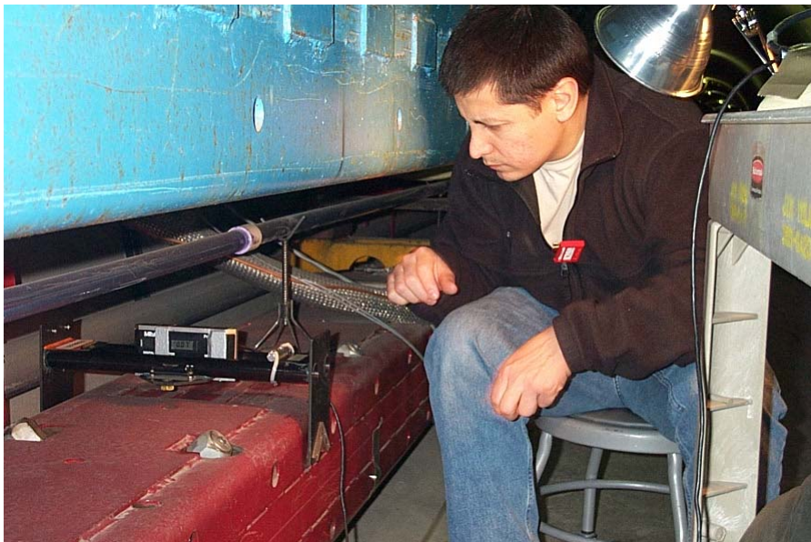
Figure 3 Digital level set on survey lugs of a Tevatron dipole
