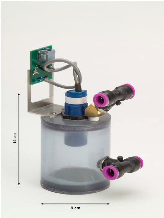
Figure 5 Fermilab Hydro Static Water Level
