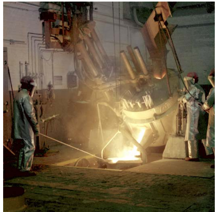
Figure 12: A heat is shown above being tapped from our 2000lb three phase electric arc furnace.
