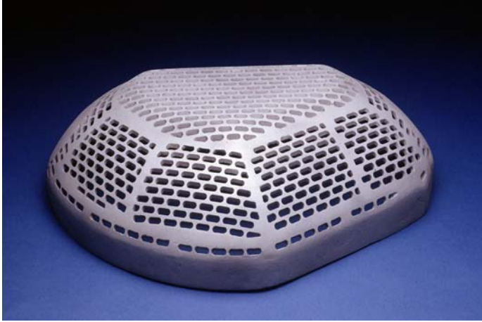
Figure 13: A P-900 hatch plate casting made using the expendable pattern casting process is shown above.
