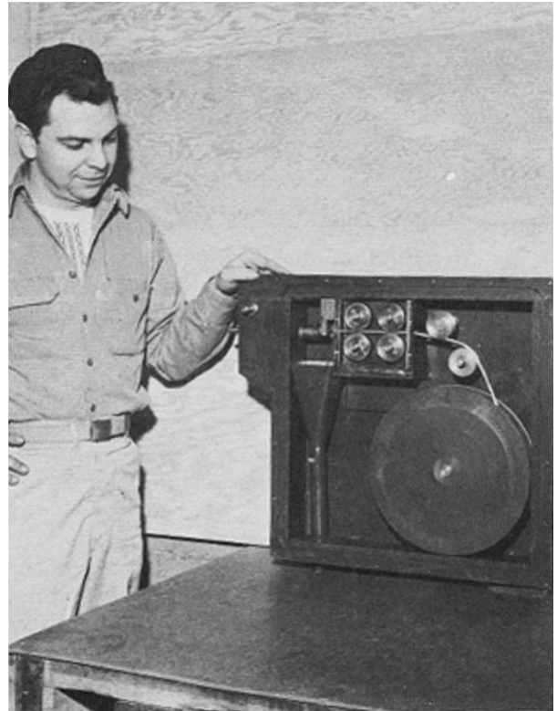
Figure 2: An automatic tin chopper/feeder mechanism is shown in the photo above, from [2].
