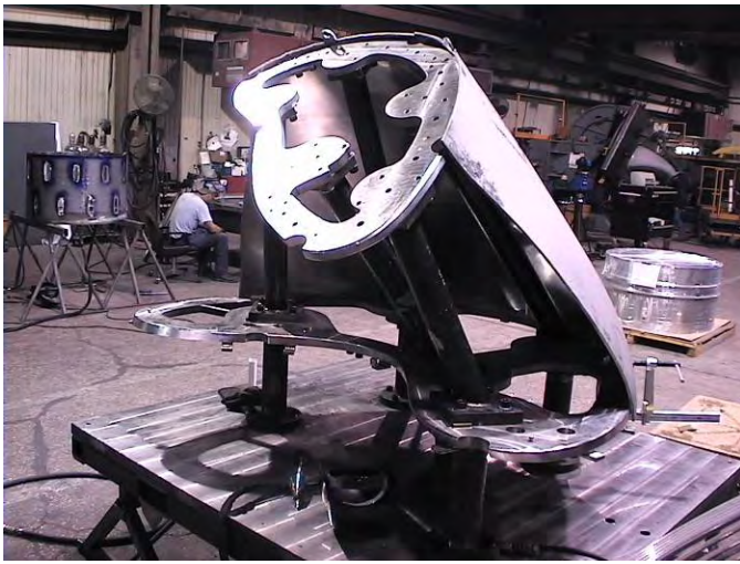
Figure 6. two panels tacked on the 60° fixture lower section
