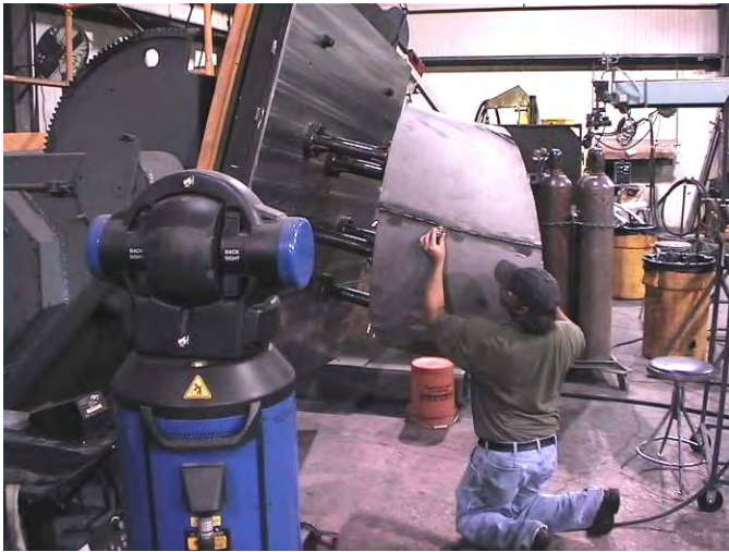
Figure 7. Final measurements being taken with a Laser Tracker
