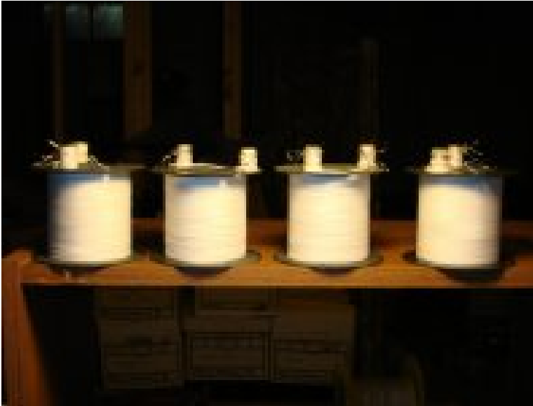
Fig. 6, Four Finished Coils after Winding and before Heat-treatment
