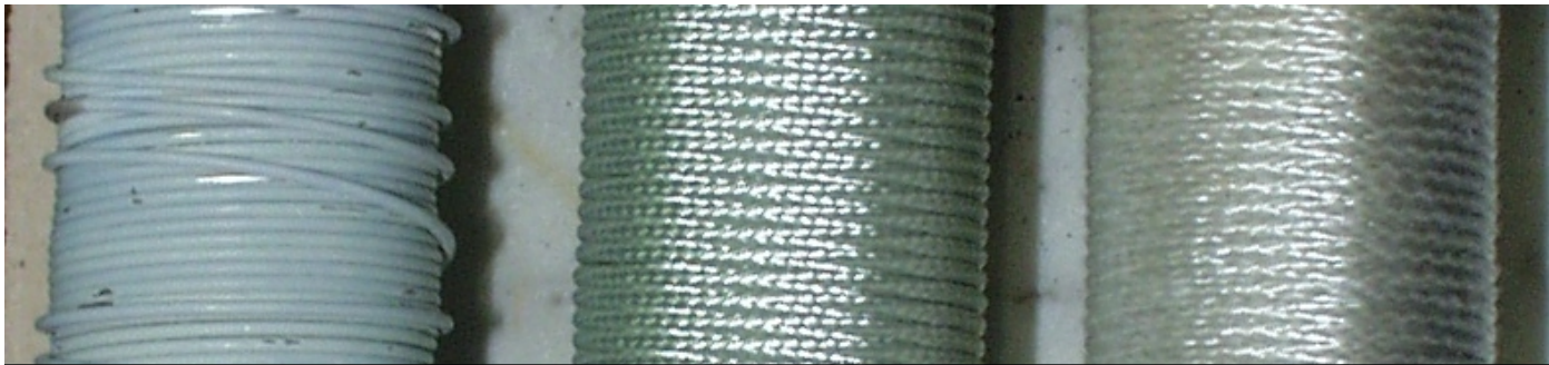
Fig. 2, Coil Insulation after heat-treatment
