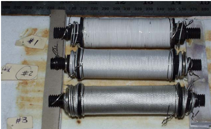
Fig. 1, 0.5" dia.x3"L. coils after winding.
