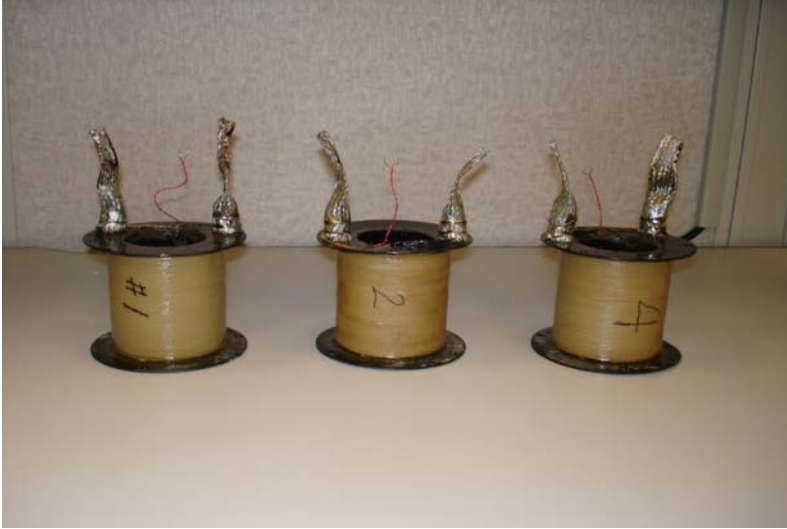
Fig. 7, Typical Coils after Heat-treatment and Epoxy VPI
