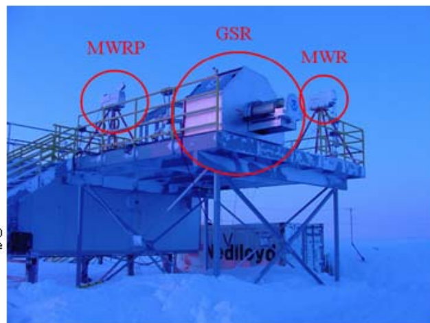
Figure 2. Photo of the deployments of the Microwave Profiler (MWRP), the Ground-based Scanning Radiometer (GSR), and the Microwave Radiometer (MWR) at the NSA/AAO during WARM04.
