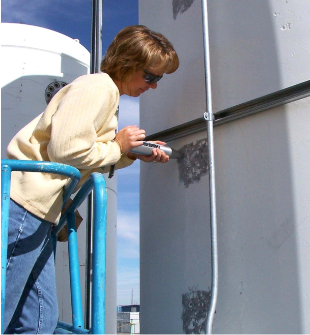
Fig. 7. Schmidt rebound hammer testing on the VSC-17 cask.
