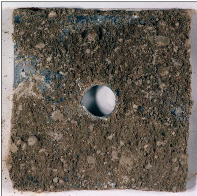
FIGURE 1 - Corroded Beryllium Coupon after Underground Exposure
