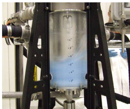
Fig.4. Mixing Annulus in V-05, 20L/min.
