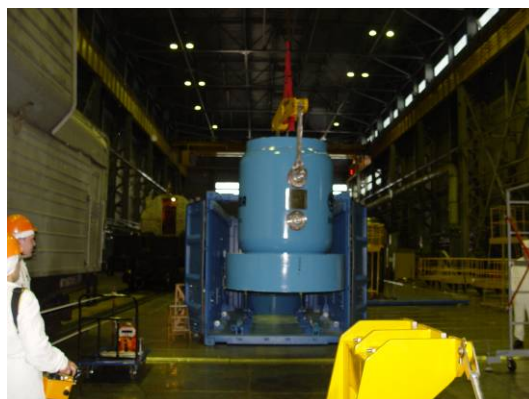
Figure 9. Cask unloading from the International Shipping Organization container in Building 855.
