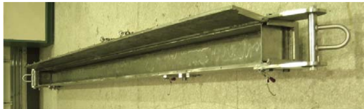
Figure 7. Rod consolidation assembly (shown with temporary lifting fixture).
