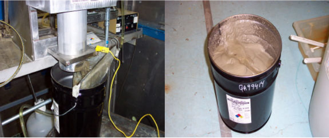
Figures 3a and 3b. Grout Mixer Testing – 5 Gallon Test
