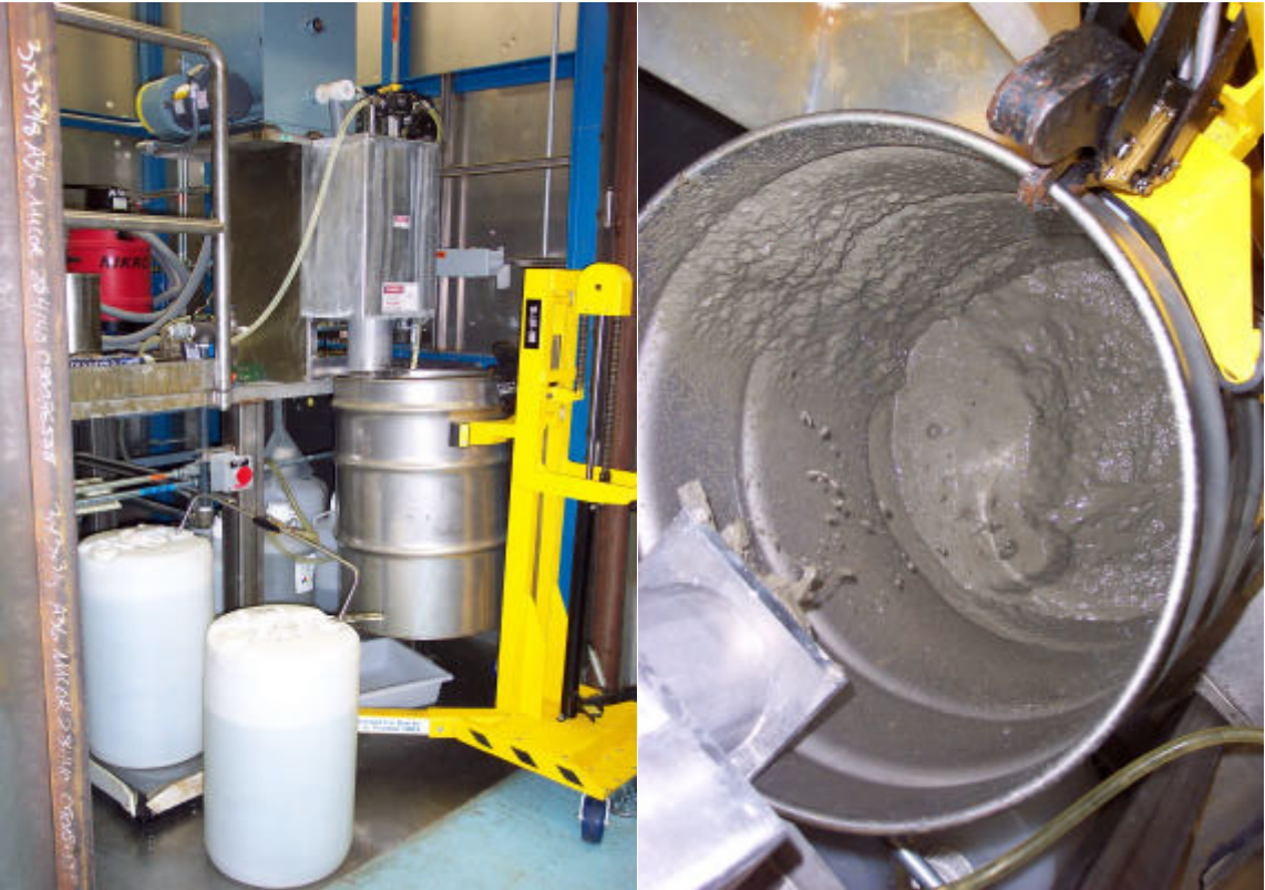
Figures 4a and 4b. Grout Mixer Testing – 55-Gallon Test
