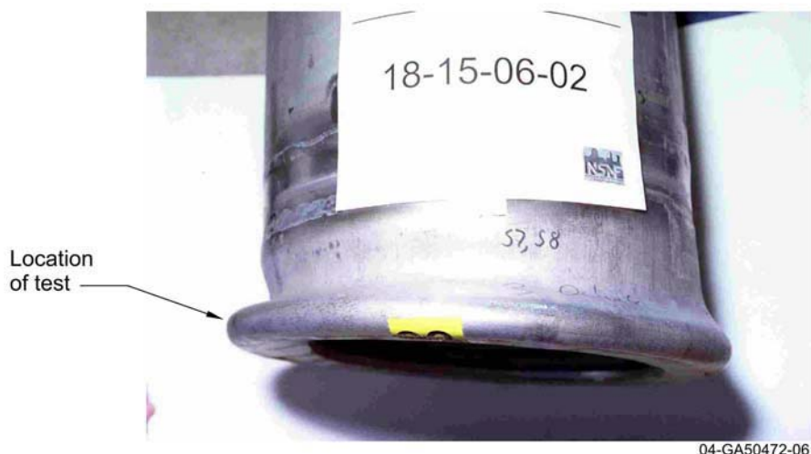
Figure A-9. Location of liquid penetrant test on representative Test Canister 02.
