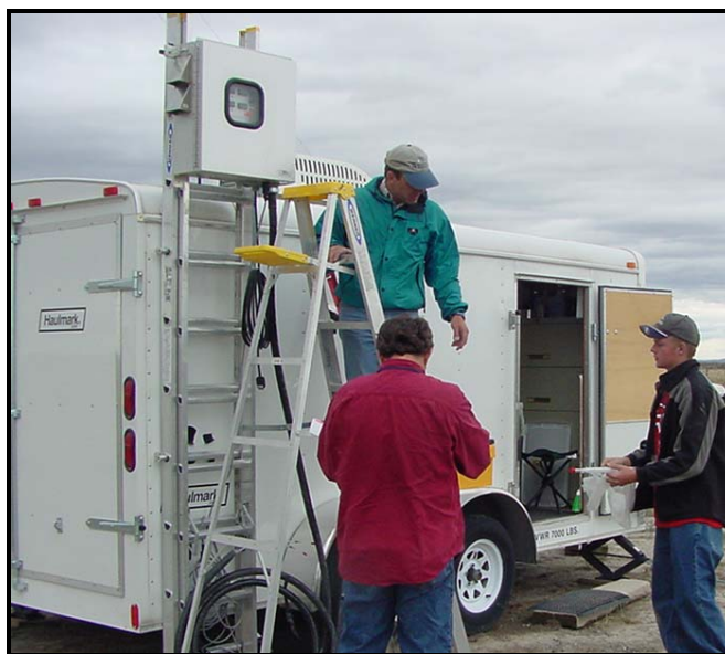
Figure 5. Tekran 1130 denuder module being installed outside the EFS instrument trailer.
