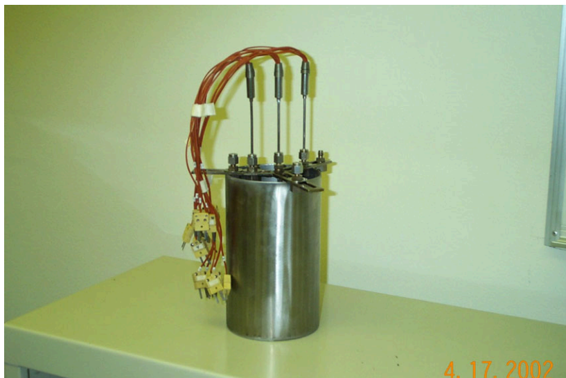
Figure 4. Photograph of a typical sludge container (1-quart nominal size) and the temperature probes utilized during vacuum-aided thermal desorption testing.
