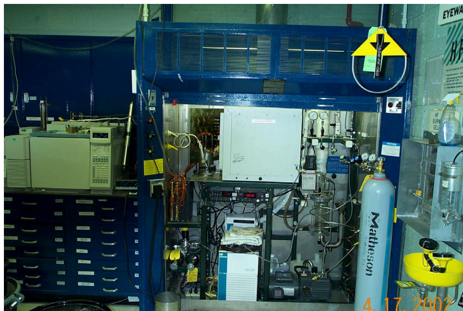
Figure 2. Photograph of experimental set-up showing the gas chromatograph and vacuum oven.
