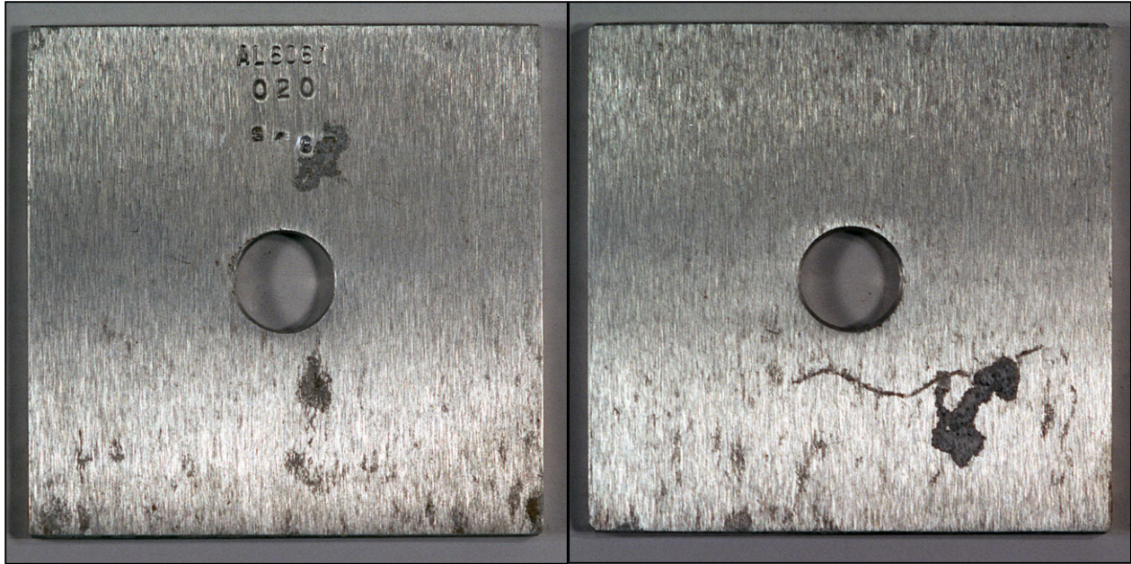
Figure 3-1. Aluminum coupon (#3497) before cleaning. 6-yr exposure at 4-ft front and back views.
