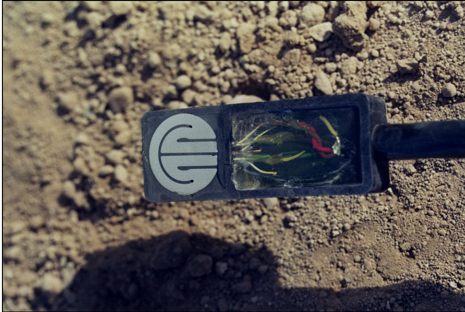
Figure 4-2. Electrical Resistance (E/R) probe. Photo shows the probe just before installation at the corrosion test berm.
