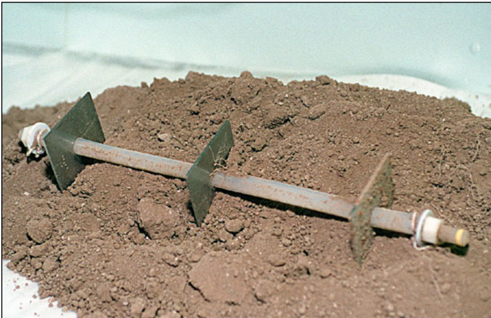
Figure 2-10. One year exposed rod from coupon array after arrival at laboratory.
