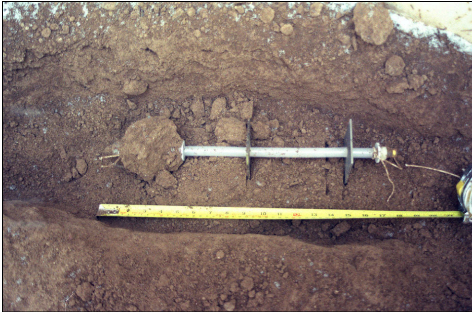
Figure 2-13. Six-year exposed rod from 10-ft coupon array. Note the beryllium sample, leftmost, with adhering soil approximately the size of a softball.
