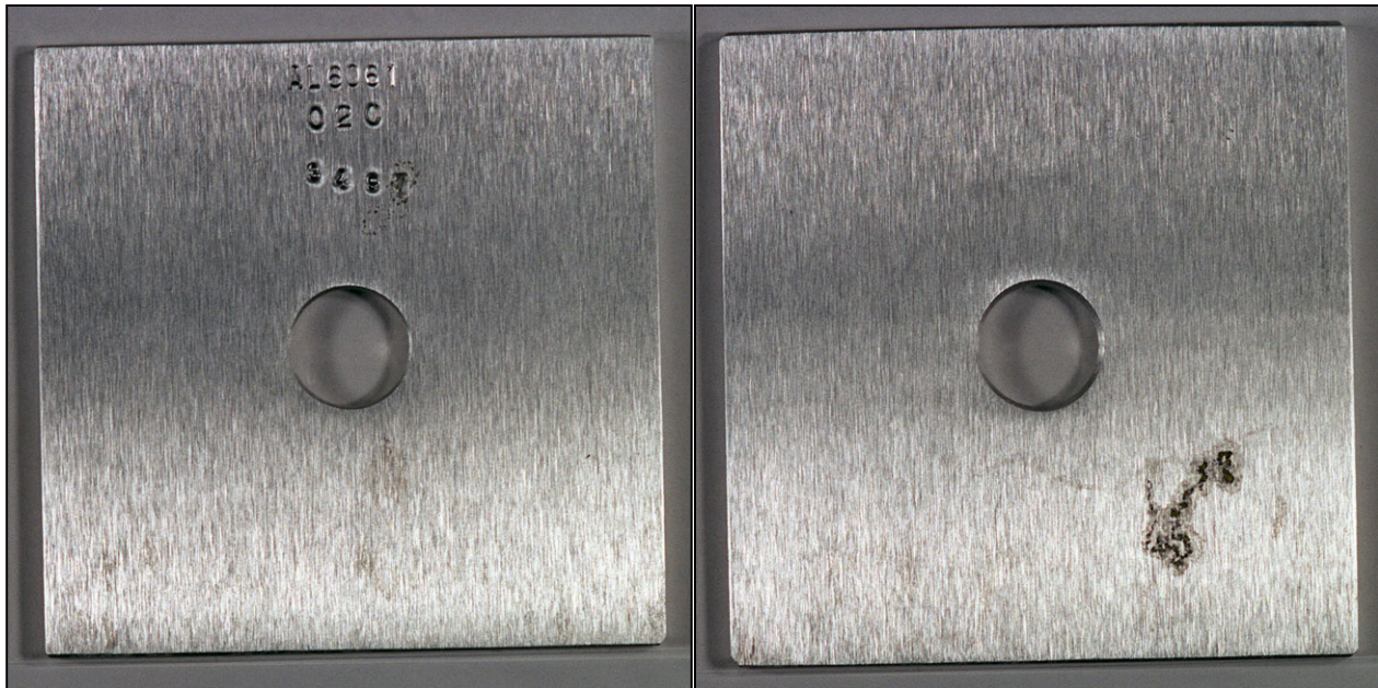
Figure 3-2. Aluminum coupon (#3497) after cleaning. 6-yr exposure at 4-ft, front and back views.
