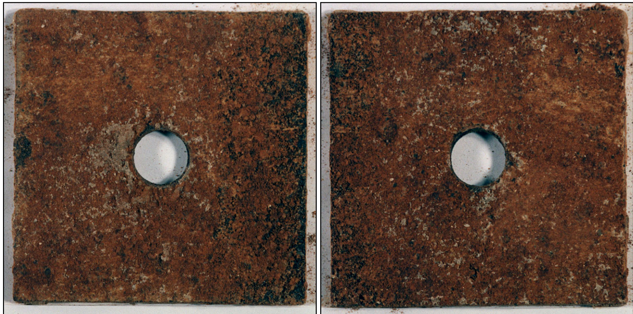
Figure 3-7. Carbon steel coupon (#3348) before cleaning. 6-yr exposure at 10-ft, front and back views.
