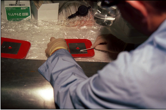
Figure 6-2. Swabbing corrosion coupon for enrichments.
