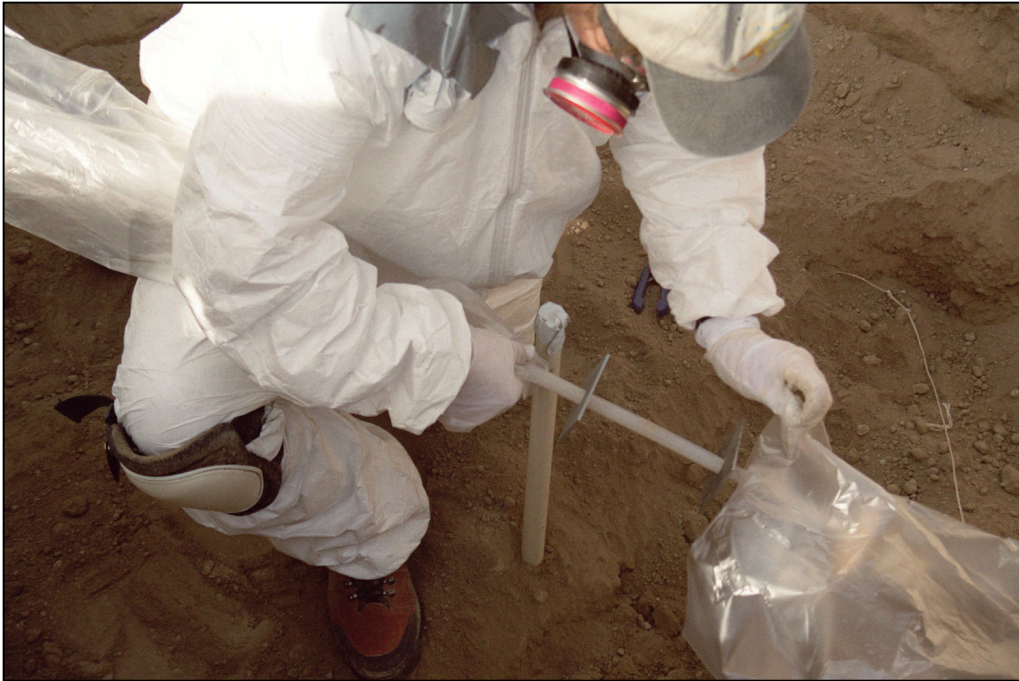
Figure 2-9. Double bagging coupons.
