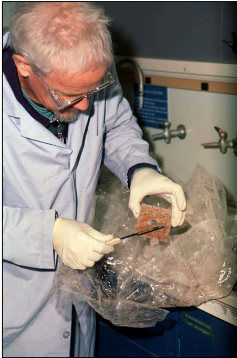
Figure 6-1. Removal of soil and loose debris for microbial testing.
