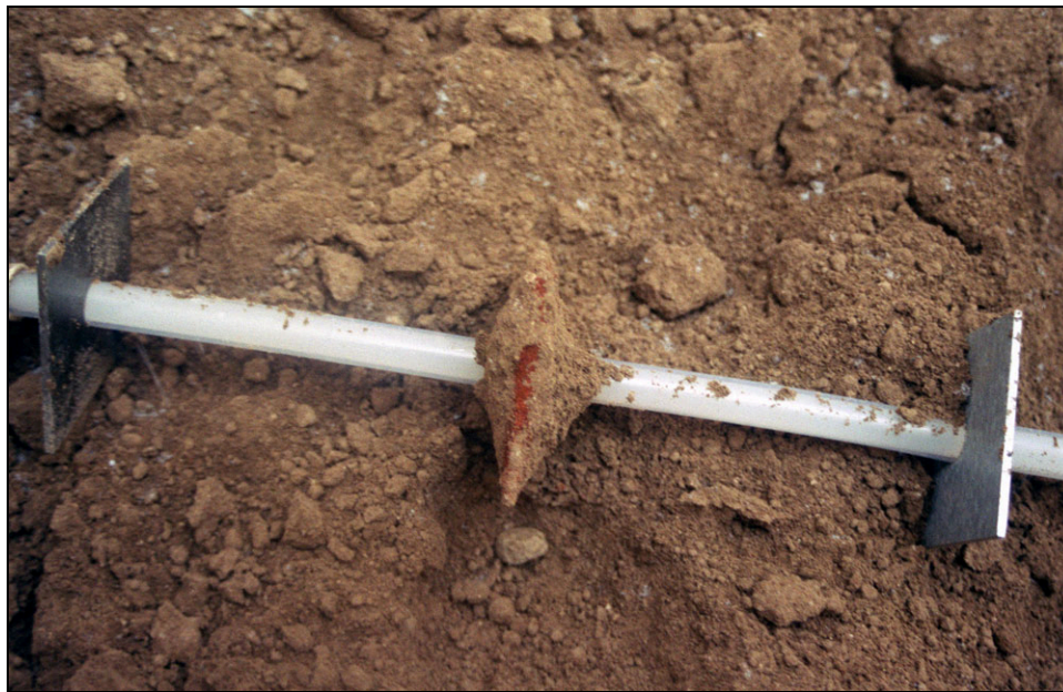
Figure 2-12. Six-year exposed rod from 10-ft coupon array. Note the carbon steel sample, centered on the rod, with adhering soil.
