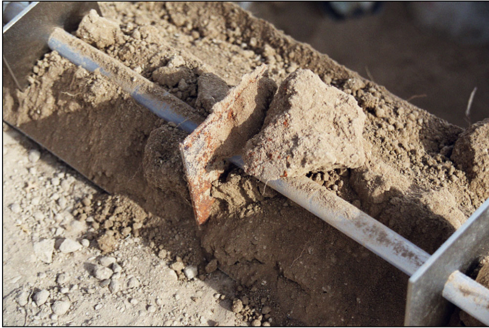
Figure 2-11. Three-year exposed rod from 4-ft coupon array.
