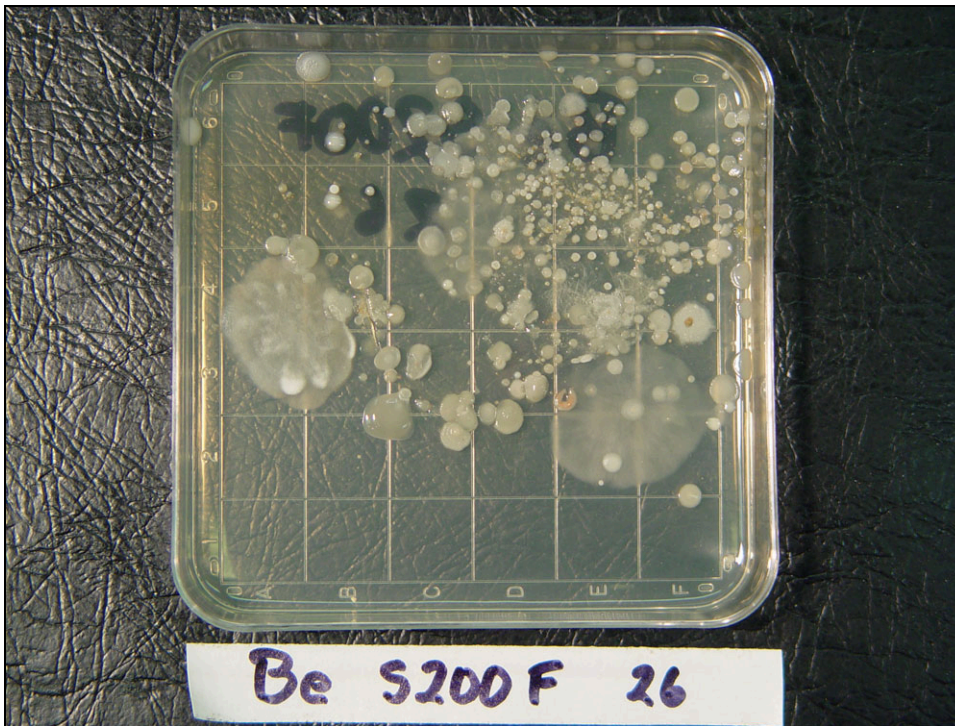
Figure 6-4. Microbial growth on contact plates imprinted from a beryllium coupon.
