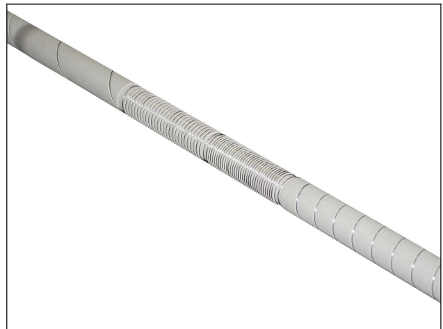
Figure 4. Photograph of steam generator with wound heater wire.
