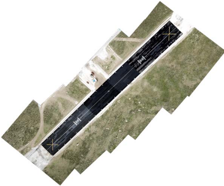
Figure 1: Georeferenced mosaic of the UAV runway at the INL taken from 8mp Canon 20D (Image-to-Image Registration).
